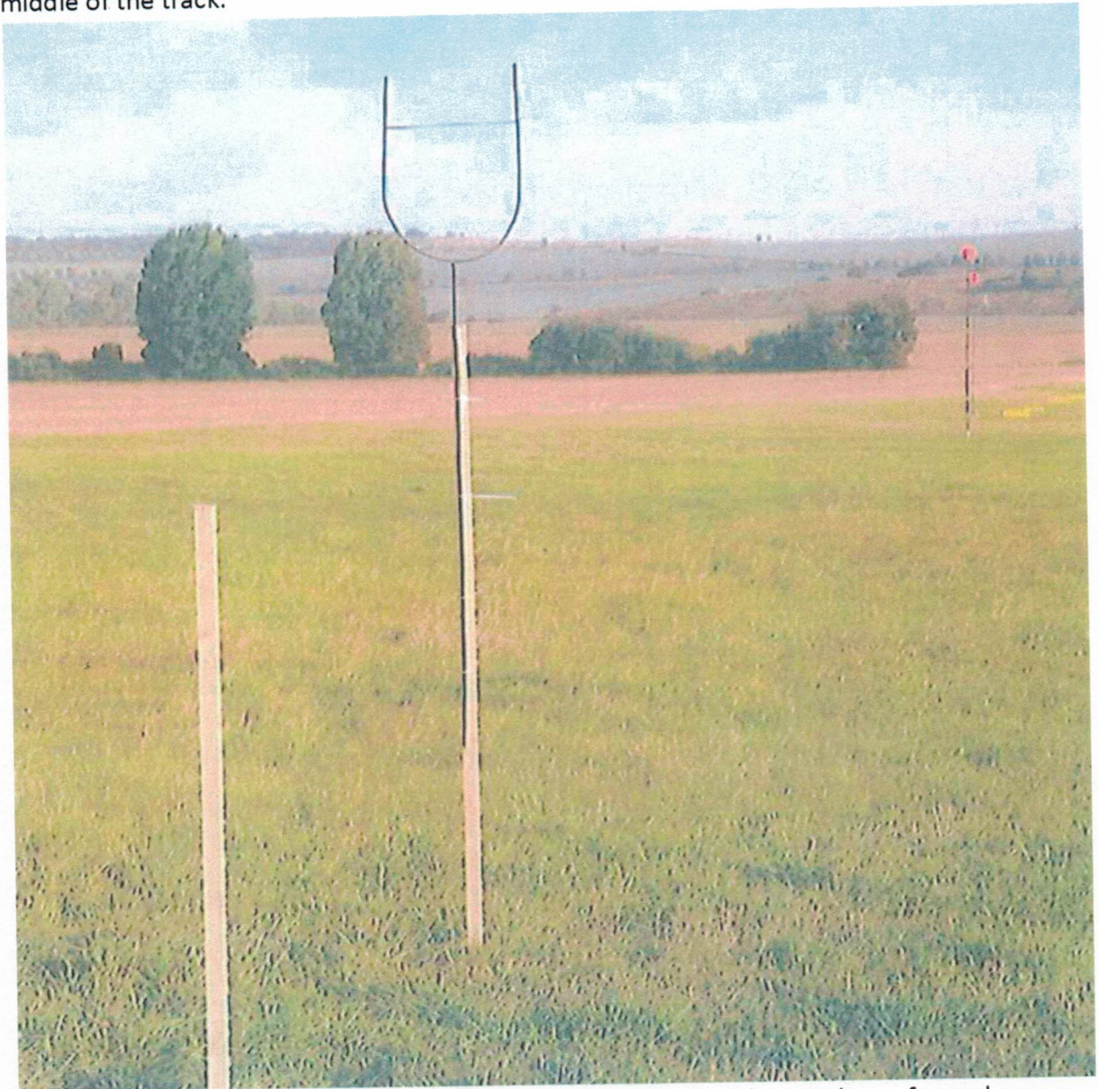
Height verification tool at the flightline with notch and bead sighter, pylons of speed course with red indicators on the tip in the background.
